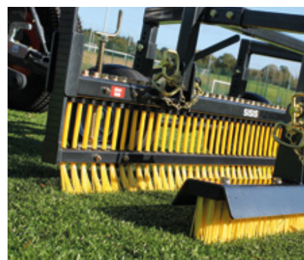
Towed frame with flexicomb and straight brush. The crossbar can be adjusted to shorten or lengthen the bristles for rubber crumb or sand infill
