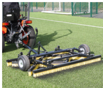
In action standing up the pile and moving the infill
