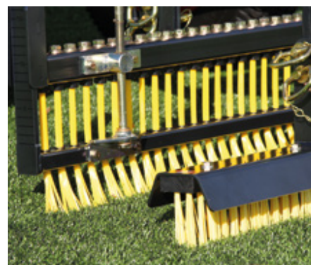
Adjustable crossbar on flexicomb alters length of bristles to meet the needs of rubber crumb or sand infill
