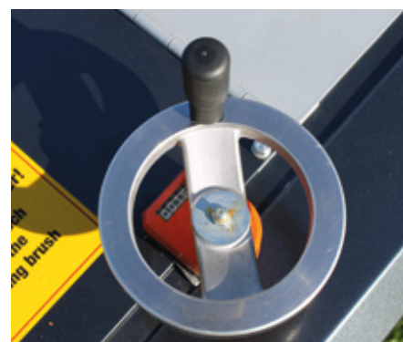
Easy to use hand wheel for working depth adjustment
