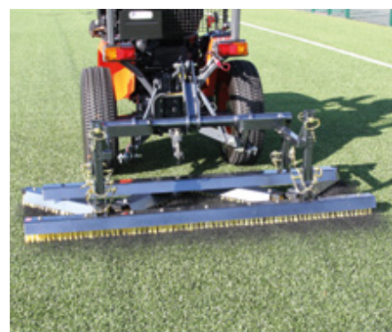
Zig Zag brush and straight brush combination at work on rubber crumb infill
