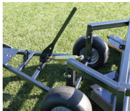
Towed frame with manual lift
