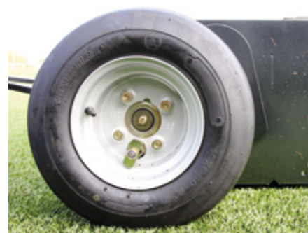
Simple "pull & twist" clutch levers on each wheel to disengage wheel drive to the brush during transport
