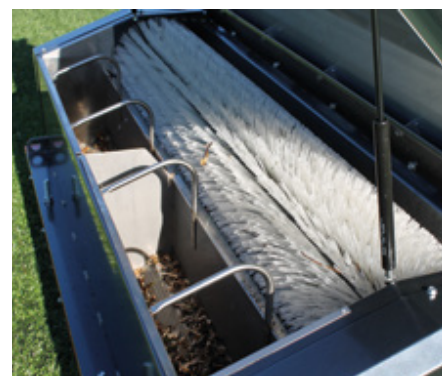
Removable sections with large debris
