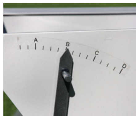
Infinitely variable spreading rate control lever
