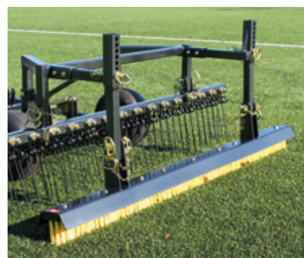
Towed frame with fine grooming rake and straight brush in action reducing compaction on rubber infill
