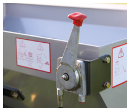
Cable control for material shut off
