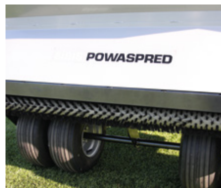
Rotating brush at point of discharge ensures even spread
