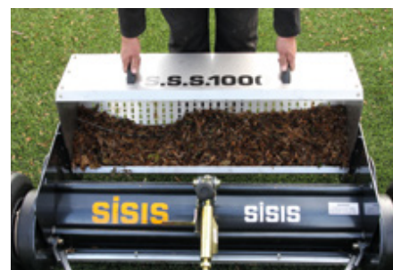
Easy-to-remove hopper and unwanted debris
