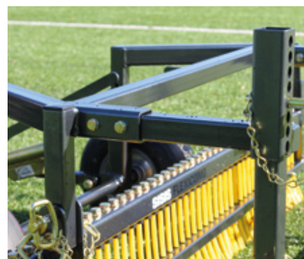
Twin implement extension arms allows a straight brush to be added to the system
