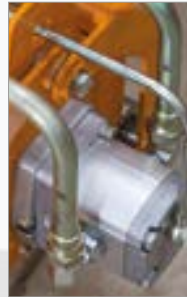
Direct Drive to reel shaft via hydraulic motor
