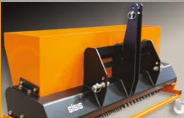
Standard cat 1, 3 point linkage for easy fitting to any tractor
