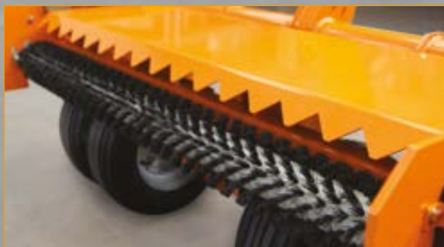
Close up of the rotating brush and oscillating plate
