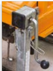
Quick, single lever tine depth setting for easy adjustment
