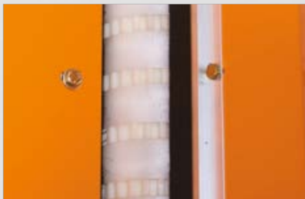
Grooved discharge roller – two discharge roller options for pure bent, rye grass/fescue
