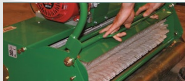
Insert new cassette onto front unit bearing stud
